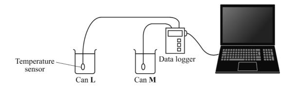
The student filled the two cans with equal volumes of hot water. He then placed the temperature sensors in the water and started the data logger. The computer used the data to draw the graph below.
