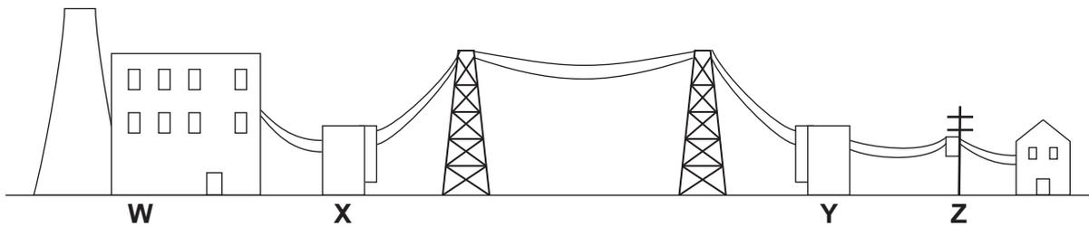
**7A** Which labelled part, **W**, **X**, **Y** or **Z**, is a step-up transformer?
