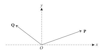
Two horizontal forces  $\mathbf{P}$  and  $\mathbf{Q}$  act at the origin O of rectangular coordinates Oxy (see diagram). The components of  $\mathbf{P}$  in the x- and y-directions are 14 N and 5 N respectively. The components of  $\mathbf{Q}$  in the x- and y-directions are -9 N and 7 N respectively.
