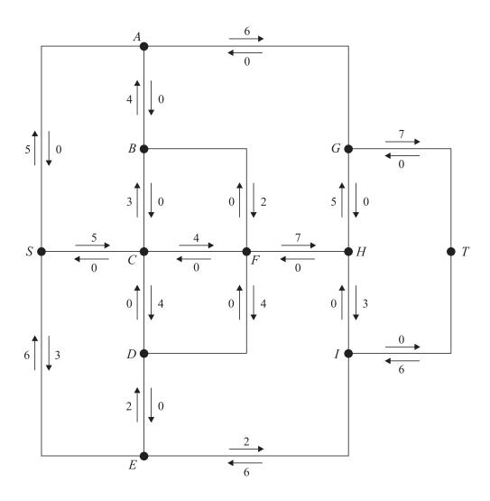
The arrows are labelled to show excess capacities and potential backflows (how much more and how much less could flow in each pipe). The excess capacities and potential backflows are measured in litres per second. Currently the flow is 6 litres per second, all flowing along a single route through the system.
